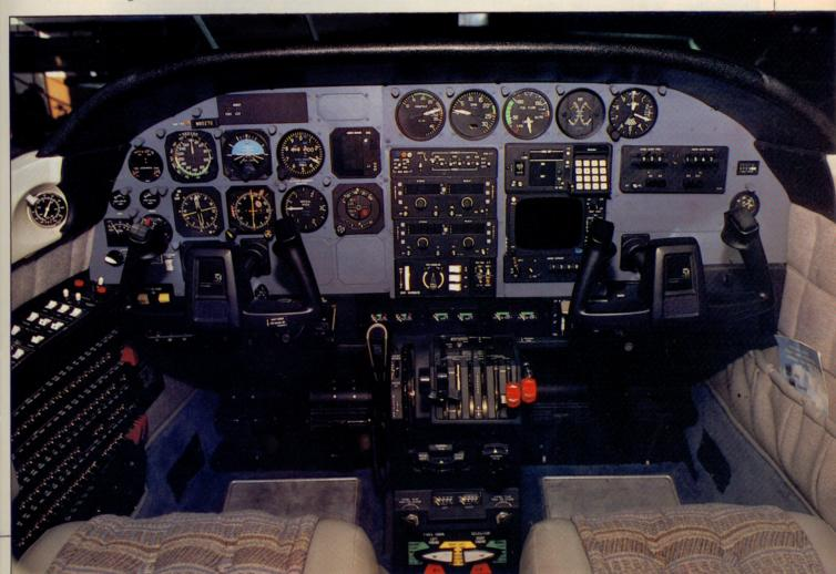
Crossfeed) are mounted on the base with the fuel gauges directly above. There is three-axis trim, with the controls on the pedestal. The engine instruments are just above the pedestal, with the manifold pressure, tachometers, fuel-flow and exhaust gas temperature gauges on the center of the panel just below the glare shield and almost directly in line with their associated controls.
